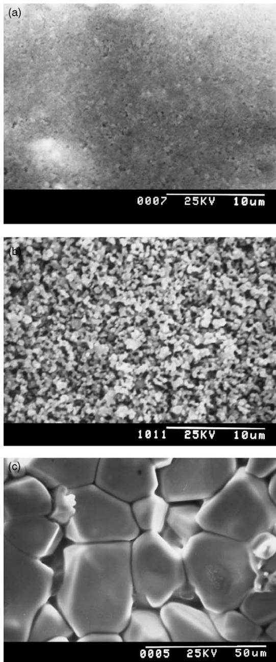
Fig. 7. SEM photos of BST thick films sintered at different temperature: (a) 800 °C, 2 h; (b) 1000 °C, 2 h; (c) 1250 °C, 2 h.
