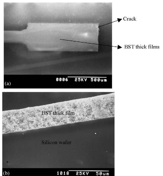
Fig. 8. SEM photos of the surface: (a) and cross section (b) of patterned BST thick film sintered at 1000 °C for 2 h.
