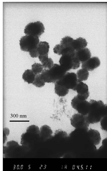
Fig. 6. TEM photo of hydrothermally treated BST powders at 200 °C for 5 h.
