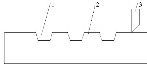
Fig. 2. Schematic diagram of tape casting: (1) grooves; (2) silicon substrate; (3) blade.
