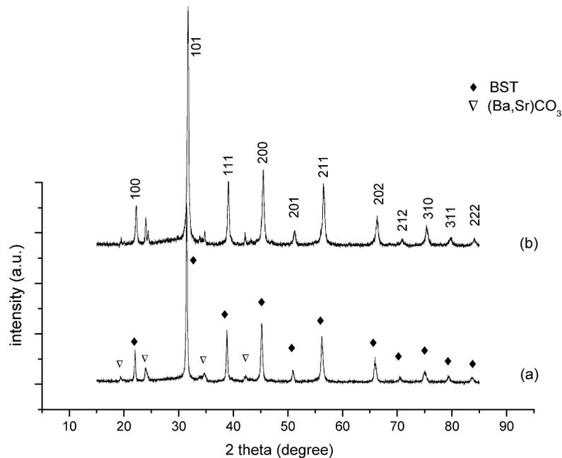
Fig. 3. XRD results of the BST powders: (a) as precipitated; (b) hydrothermally treated at  $200^\circ\text{C}$  for 5 h.
