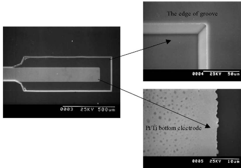
Fig. 1. The SEM photos of groove with patterned bottom electrode in the silicon substrate.
