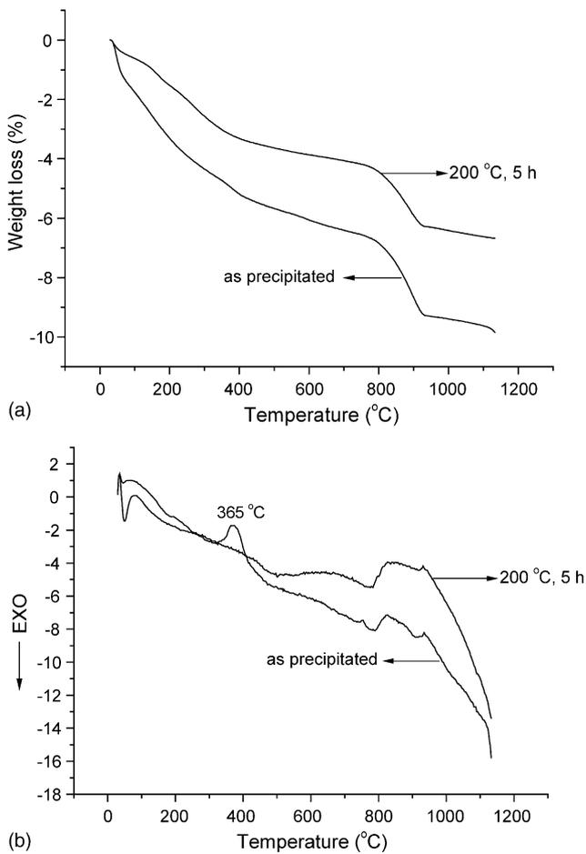
Fig. 5. TG (a) and DTA (b) analysis of as precipitated and hydrothermally treated BST powders (200 °C for 5 h).
