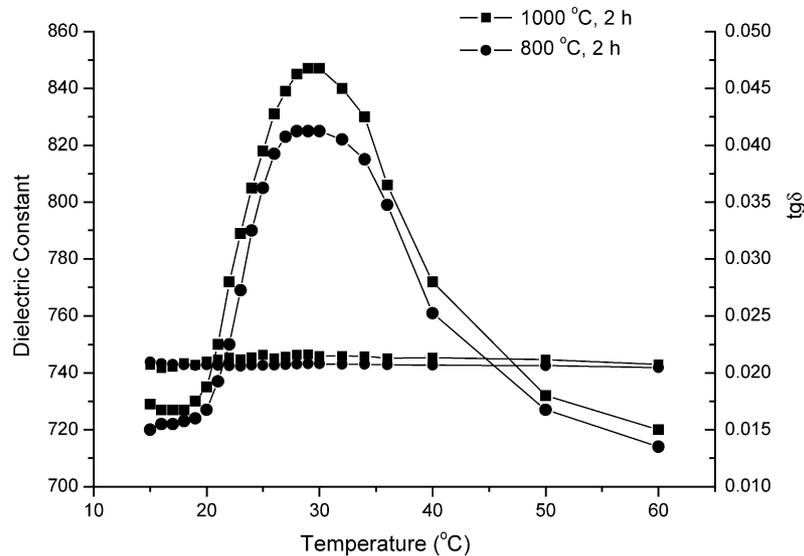
Fig. 9. Temperature dependent of dielectric constant of BST thick film (1 KHz) sintered at 800 and 1000 °C for 2 h, respectively.
